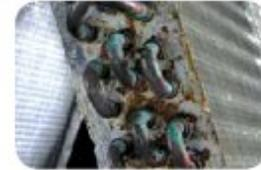
Copper tube and galvanized steel tube sheet after 500 hours in a controlled corrosive environment.
